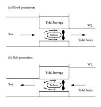
The Power Generated (Watts) = (Turbine's efficiency  $\times$ Density of Water  $\times$  The swept area of the turbine  $(m^2)$ [The velocity of the flow]  $^3$ )/2.
